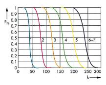
FIG 9 Eight-channel receiver: probability  $P_N$  of at least k hits in  $N=10^4$  repeated attempts with mean number  $\bar{n}$  of valid intercept attempts during one hop interval
