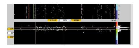
FIG 3 Detection of two FH transmitters near noise limit with Digital Scanning Direction Finder DDF01S in same frequency band 6784.1 to 6896.8 kHz marked by vertical cursor lines. In waterfall display (upper display window) two transmitters cannot be distinguished, in azimuth versus frequency display in lower window and azimuth histogram right it can be seen that two FH transmitter signals arrive with azimuth difference of 36°.
