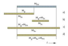
FIG 5 Frequency bands of hopper and receiver:
