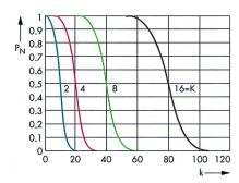
FIG 10 Receiver with K parallel channels,  $\bar{n}=1$ : probability  $P_N$  of at least k hits in  $N=10^4$  repeated attempts
