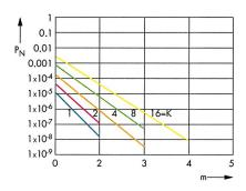
FIG 11 Receiver with K parallel channels,  $\bar{n}=1$ : probability  $P_N$  of at least m hits in N=10 repeated attempts
