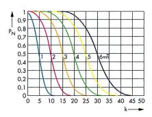
FIG 8 Single-channel receiver: probability  $P_N$  of at least k hits in  $N=10^4$  repeated attempts with mean number  $\bar{n}$  of valid intercept attempts during one hop interval
